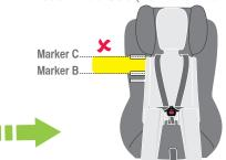
Move to the next form of child restraint when the child's shoulders reach the upper shoulder height marker C.
