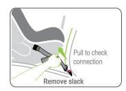
H. Push downwards on the seat to compress the seat into the vehicle. Whilst pushing into the seat, pull on adjuster strap to remove all slack and tighten the ISOFLEX strap. Repeat for the adjuster strap on the other side of the restraint. The two tension indicators will show green indicating minimum tension has been applied.
