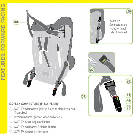
31. ISOFLEX Connector32. ISOFLEX Adjustment strap33. Top Tether Assembly
