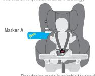
Rear facing mode is suitable for shoulders below the Lower Height Marker (A)
