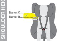
Forward-facing mode is suitable for shoulders above shoulder height marker B but not below marker A.
