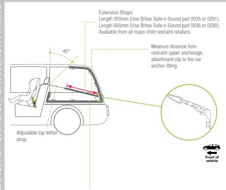
The shaded areas of this diagram illustrate the possible locations of the upper anchorage point (car anchor fitting). Within each shaded area is an upper anchorage point showing the correct way to install the fitting. Ensure the upper anchorage point is aligned as illustrated unless stated otherwise in the vehicle owner's handbook.
