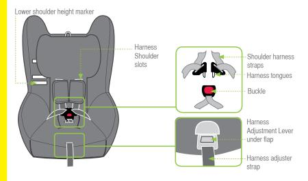
Adjustment of the headrest automatically adjusts the harness shoulder strap position. If the headrest has side wings they should be just above the child's shoulders. If there are no side wings, the shoulder straps must be in the slots which are nearest to the child's shoulders, but not more than 25 mm below the child's shoulders.
