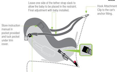
With baby installed, pull to remove all slack do not over tighten causing the seat to lift.
