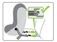
F. Push downwards on the seat to compress the seat into the vehicle. Whilst pushing, pull on adjuster strap to remove all slack and tighten the ISOFLEX strap. Repeat for the adjuster strap on the other side of the restraint. The two tension indicators must show 'green' indicating minimum tension has been applied.
