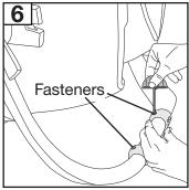
Use one hand to apply pressure and hold the bracket closed. Then use your other hand to engage and firmly tighten both fasteners into the bracket with the hex wrench.
