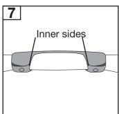
The fasteners are tight when the inner sides of the bracket are flush.
