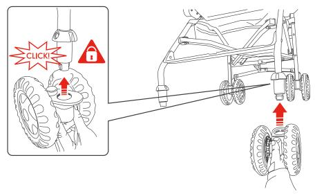
B To remove each front swivel wheel assembly, Use long nose pliers and squeeze both sides of the inner tube and pull wheel assembly out.
